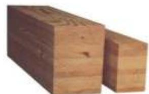
gives the glulam strength in one direction and for this reason glulam is predominantly used for structural beams.
