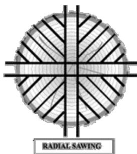
close to radial sections because the rings are nearly at right angles to the face of the boards. A summary of the main environmental and technical benefits of radial sawing include: more timber out of each log, higher value products from younger trees, timber products with consistent growth rings, and more stable wood, less likely to move after processing.
