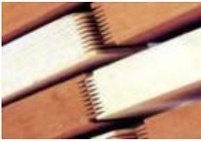
**Finger Jointing** is employed for maximizing use and reduction in wastage of wood along with for imparting improved aesthetic value.
