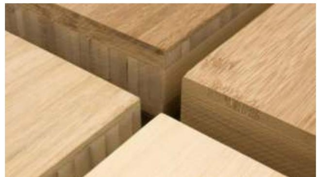
is surprisingly strong, with up to three times the structural capacity as normal timber. Despite this, there remain some concerns about the bamboo's resilience, as it decays more quickly than wood if not treated with the right preservatives.
