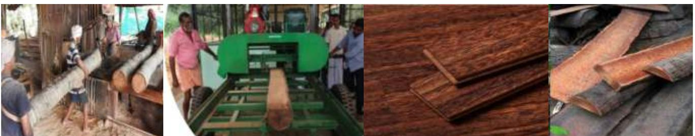
light/general purpose portable sawmill, a mini mill, a breast bench with light weight carriages and a chainsaw with guide attachments. Problems of sawing coconut logs are similar to the ones encountered by saw millers when using high density species of tropical hardwoods.
