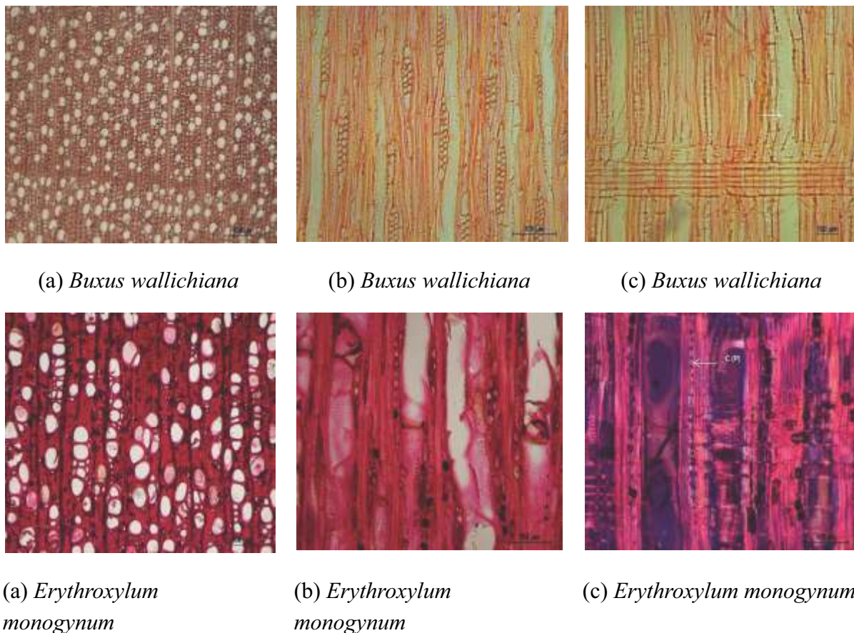
Figure 2: Anatomical structure of adulterants of sandalwood (a) cross-section (b) TL section, (c) RL section (Symbol ‘C’ in photomicrographs indicates the location of crystals)
