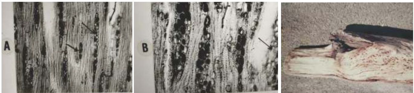
Fig. 3. Anatomy of Pin hole variety of sandalwood A. Biseriate medullary rays B. Multiseriate medullary rays C. Sandal billet with pin holes
