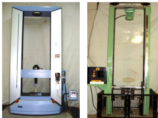
Fig.2 Timber testing machines for evaluating mechanical properties of wood (a) Universal timber testing machine (UTM, Shimadzu), (b) Impact bending machine
