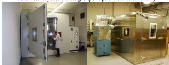
Fig.4 Test chambers for (a) environmental and (b) VOC & formaldehyde emission testing (Sources: https://www.camal.ncsu.edu ; https://www.tuv.com )
