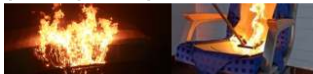
Fig.3 Flammability testing of furniture (Sources: https://www.stc.group ; https://www.rst-labs.com )
