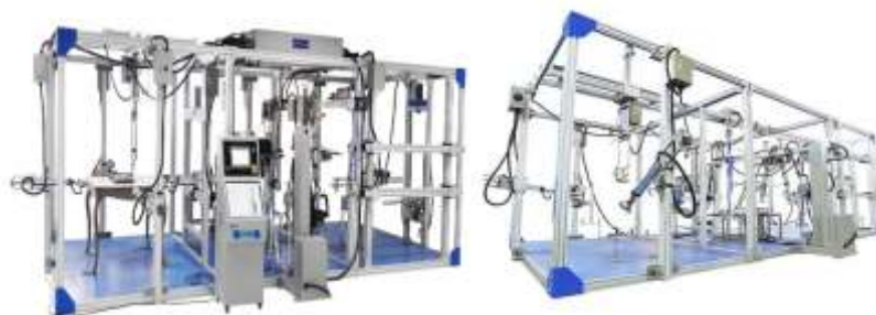
Fig.1 Furniture universal test machines (Source: https://www.haidatestequipment.com )
