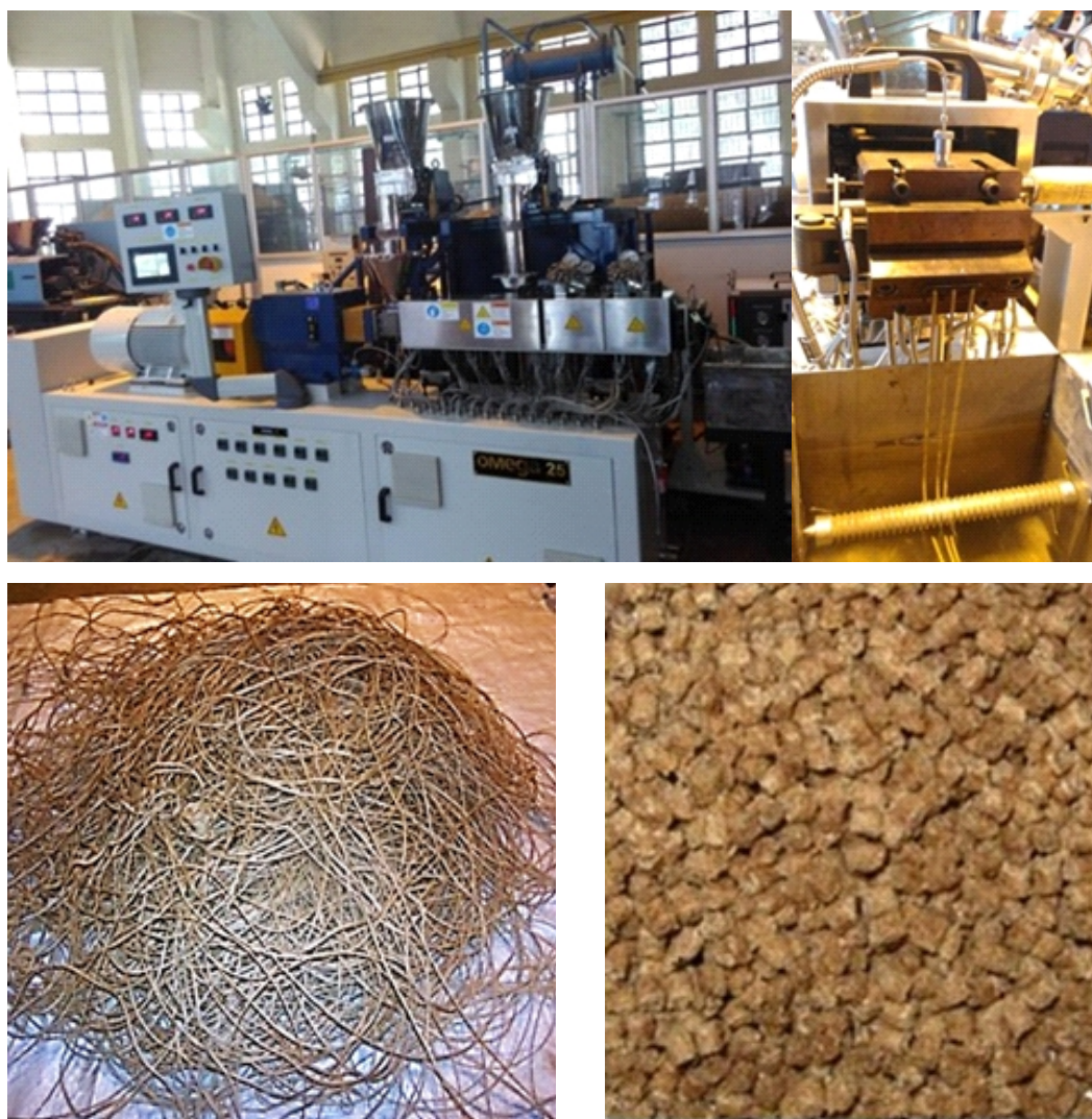
Fig.3: Lantana-polypropylene composite strands (left) and pallets (right)
