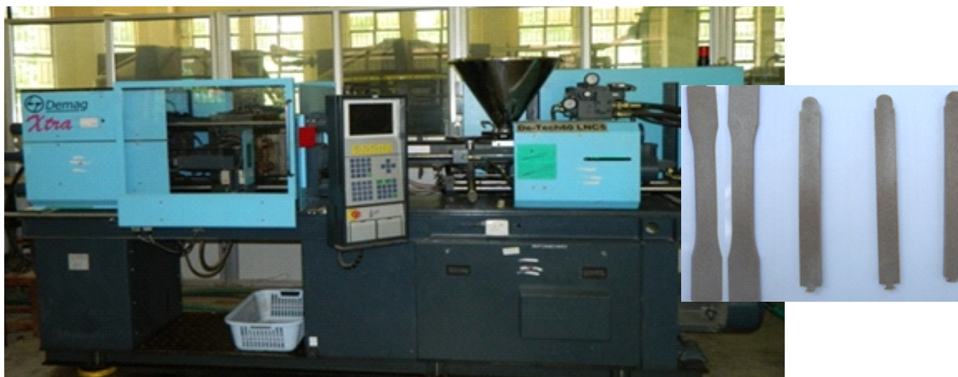
Fig 4: Injection moulding of Lantana-PP composites
