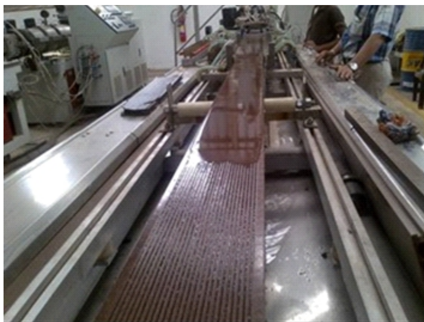
Fig. 5: Profile extrusion of Lantana-PE composites
