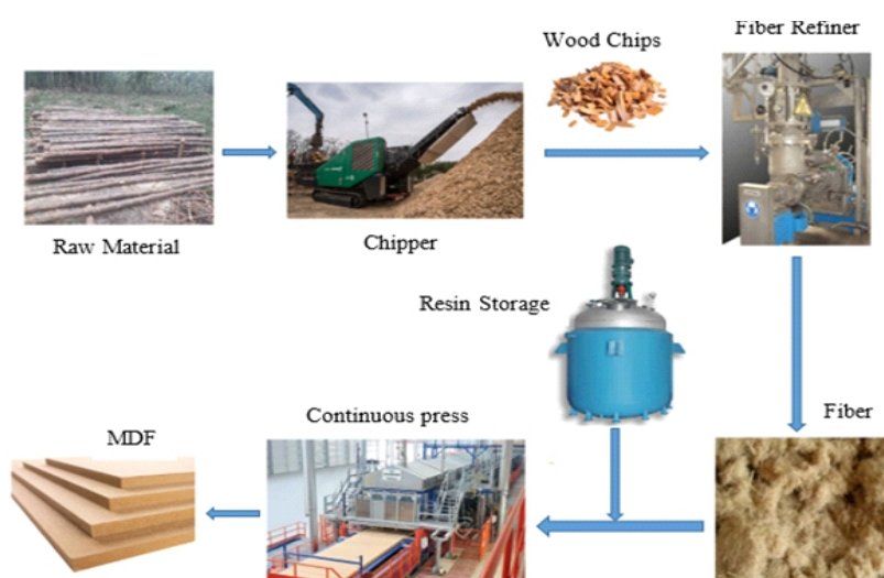
Fig 3. Pictorial flow chart of MDF manufacturing
