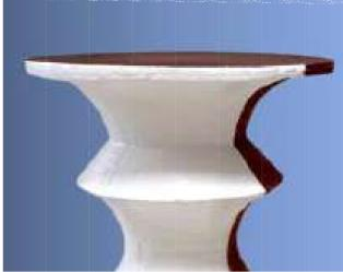
Bacteria can be used to create sustainable biocomposites with a wide variety of properties from wood waste. Picture No. 3: Composite block made out of wood and microbe (as adhesives). Picture No. 4: Furniture made of the new material. This is in complete contrast to many materials previously made of wood, which involve processing petrochemical-based adhesives that are then considered hazardous waste. (Picture Source: Johannes Falkenstein, University of Freiburg)
