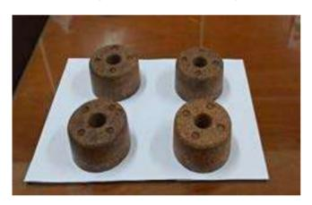
**Fig-1**. Wooden core plugs developed at Institute using wood dust and bagasse pith
