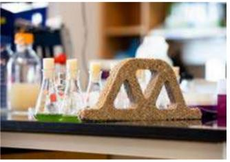
Bacterial species amalgamate different materials. Picture No. 5: Pieces of the brick, being "grown" in molds. Picture No. 6: The bricks are made from sand, hydrogel, and Synechococcus cyanobacteria (Picture Source: CU Boulder College of Engineering and Applied Science)
