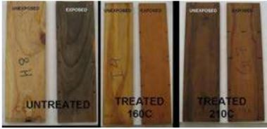
**Fig. 3.** Comparison of colour in unexposed and exposed specimens of after 2100 hrs of accelerated UV weathering. The unexposed and exposed samples belong to the same piece cut from middle of thickness of the same specimen.
