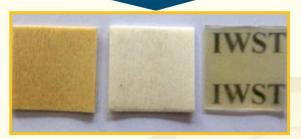
Natural wood (Left most), Lignin modified wood (middle) and Transparent wood (right most) placed on a paper with letters "IWST"
