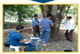
Measurement of hollowness in a tree using ultrasonic detector
