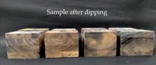
Figure 3. Swelling test sample of rubber wood glulam.
