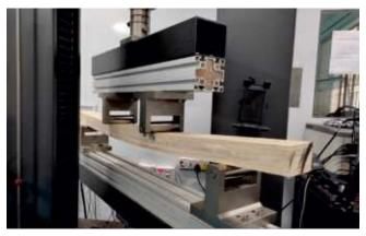
Figure 4. Bending test sample of rubber wood glulam
