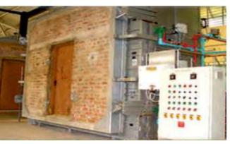
Figure 1. Fire door testing setup.
