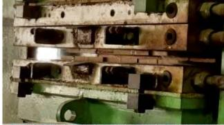
Figure 7. Assembly layup for CLT under pressure in hydraulic press.
