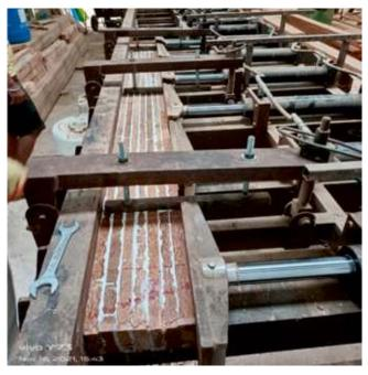
**Figure 1.** The 30 feet Hydraulic Beam Press.
