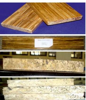
Figure 2. BSL prepared using crushed strands of B. bamboo bonded with PF adhesive.
