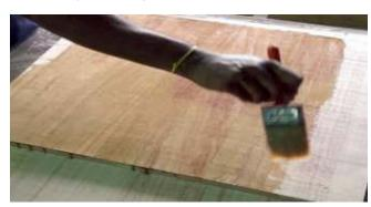
Figure 6. Adhesive application for middle layer of CLT.
