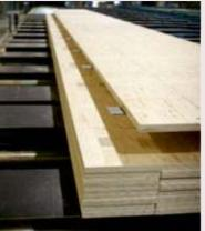
**Figure 2.** (a) Prepressed LVL billet of long span.
