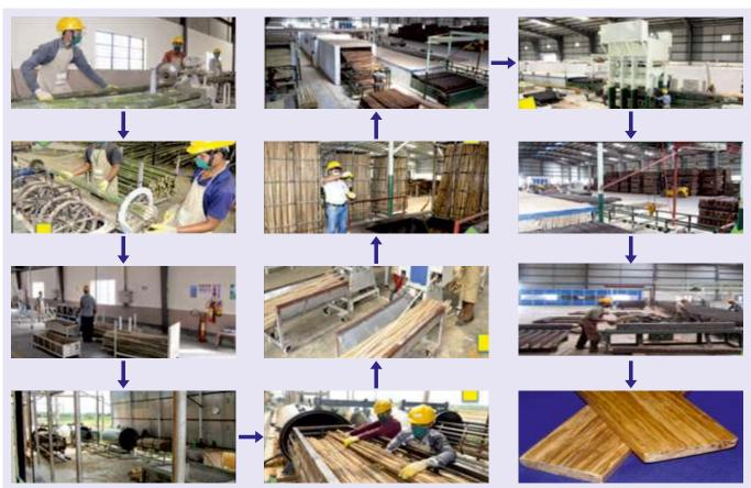
Figure 1. Flow chart of the process for manufacturing bamboo strand lumber.
