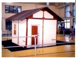
Figure 1. Testing of prototype bamboo House on shake table under seismic simulation
