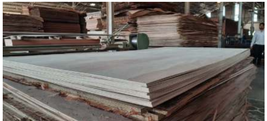
Plywood with Silver Oak commercial face veneer.
