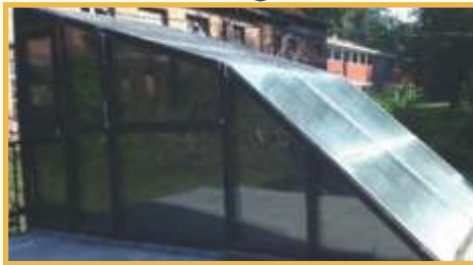
Head based storage Solar Kiln
