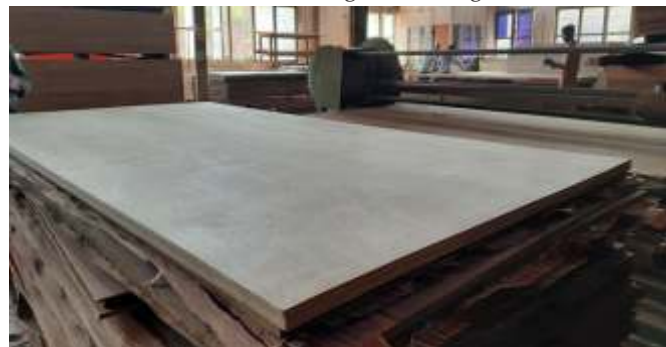
Fig. 5 Plywood made in combination of silver oak and balanji species at Industrial trial
