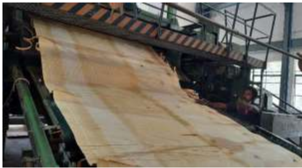
Log being cut to veneer and collected Dried Veneer
