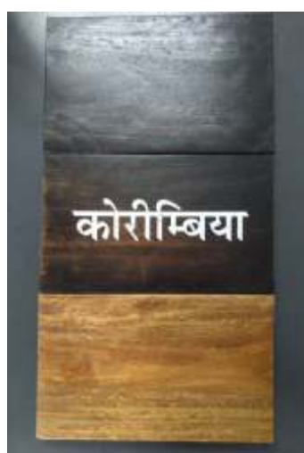
Figure 5: Polishing of Corymbia wood with black stain, walnut stain, lac stain showing good grain (in order of top to bottom).
