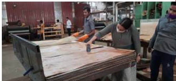
Fig. 4 Moisture checking of glue coated Balanji veneers during assembling
