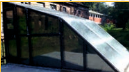
Head based storage Solar Kiln
