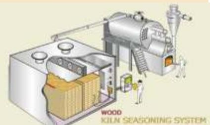
vacuum-based convection-heated wood dryer for fast and efficient drying of Indian timbers were done and further design improvements were made for improved efficiency; . seasoning studies on important species of bamboos for handicrafts using dehumidifier and Vacuum kilns, vacuum press drying studies on Melia composite were successfully attempted.
