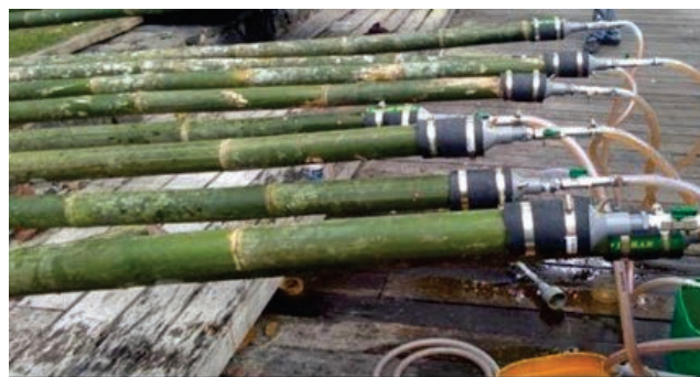
Fig. 3: Treating green bamboo by Boucherie Process
