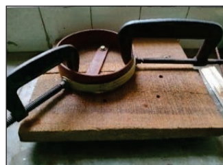
Bamboo strip on frame after Microwave treatment
