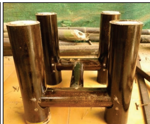
Fig. 3B manufacturing of bamboo frame for table.
