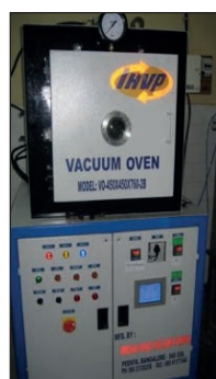
Fig. 1 Vacuum oven used for heat treatment of bamboo in laboratory
