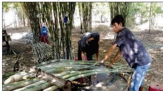
Bamboo straightening by baking over an open fire
