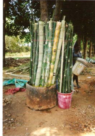
Sap-displacement of Bamboo
